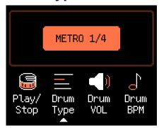
Rotate the VALUE knob to change the drum machine rhythm pattern (connect to the mobile app for more rhythm patterns).
