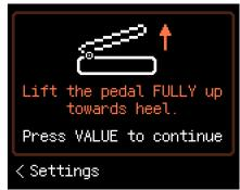
Raise the pedal completely, then press the VALUE knob to confirm.
