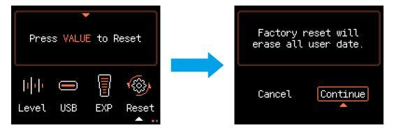
Press the VALUE knob to enter the factory reset interface. After selecting "Continue," the system will execute the factory reset operation. This action will clear all previously edited presets and personalized settings, restoring the device to its initial factory state.
