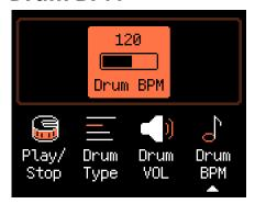
Rotate the VALUE knob to change the drum machine playback speed.
