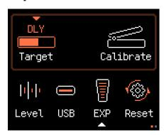
Target: Settings for the control target of the external expression pedal, selectable options are None, FX, DRV, AMP, MOD, DLY, RVB, VOL.
